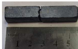
Figure 3.8: Materials consolidated with 50WC-50Cu cycle1 conditions.
