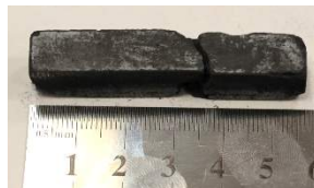
Figure 3.1: Material resulting from consolidation under 75WC-25Cu cycle1 conditions.
